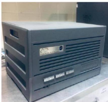
**Fig. 1.** A manual TLD Reader model of 7103-Plus
