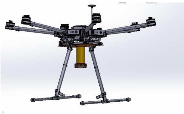
Fig. 5. The 3D Model of the holder structure assembled on the drone.
