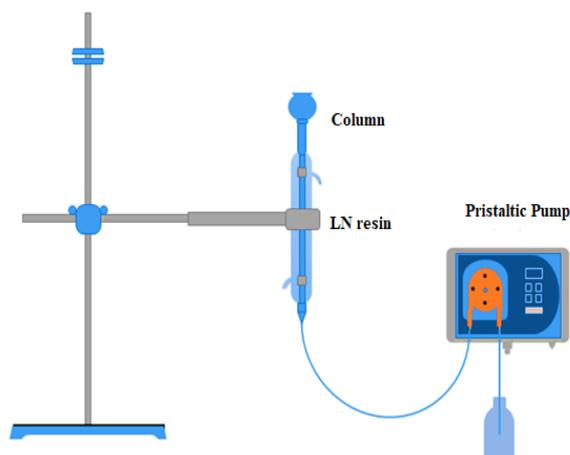
**Fig. 1.** Extraction chromatography separation system.
