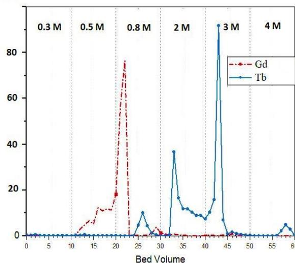
**Fig. 2.** Separation profile of Tb and Gd on the Ln resin based on ICP analysis.
