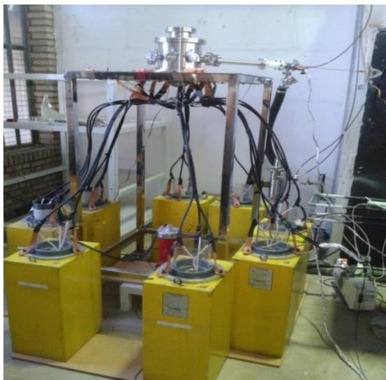
**Fig. 2.** Plasma focus 2.5Kj and its capacitors.
