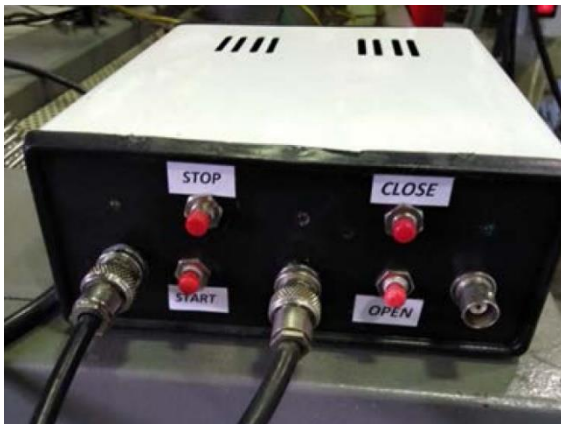
Fig. 5 the electronic control unit of the beam chopper.
