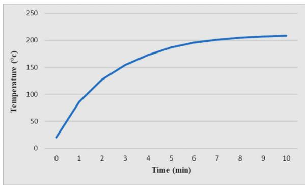
**Fig. 3.** The trend of temperature change over time in the presence of coolant.
