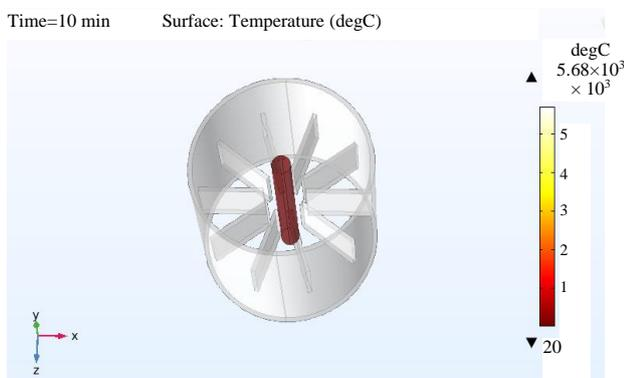
**Fig. 4.** Magnetron temperature rise over time without cooler.
