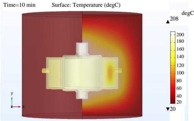
**Fig. 2.** Temperature changes over a period of 10 minutes in the presence of coolant.
