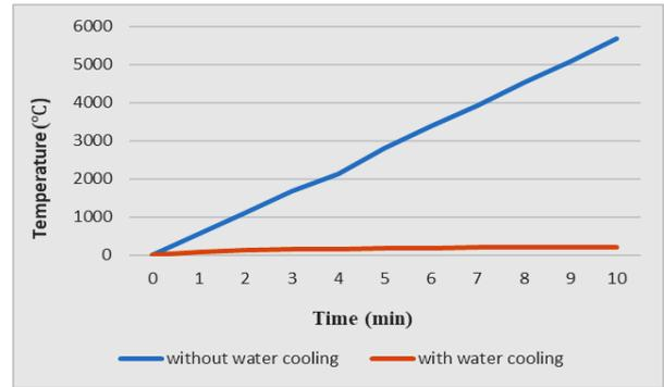
**Fig. 5.** The process of changing the temperature of the magnetron over 10 minutes. Red diagram: in the presence of a water cooler, blue diagram: without the presence of a cooler.
