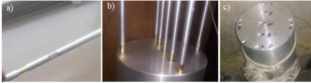
Fig. 4. Aluminum phantom of a) aluminum rod b) the rod loading inside the phantom c) the phantom full view.
